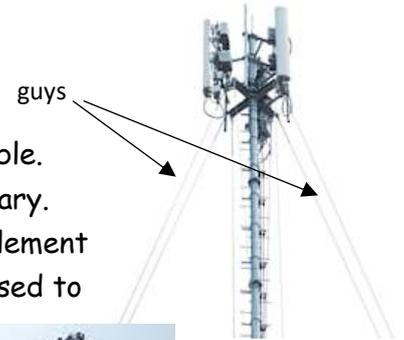
The next cell phone tower is called a **lattice** tower. It is made of criss-crossing parts. The frames consist of a series of stiff metal **columns** and **beams** that are welded or bolted together.
